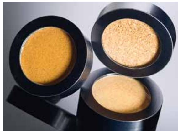
Sample cell of dried distillers grains for spectroscopic analysis.
