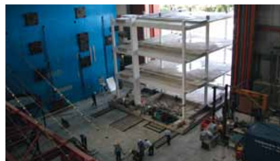
A 4-storey full scale model tested in the JRC's European Laboratory for Structural Assessment (ELSA) to study the effectiveness of seismic retrofitting of reinforced concrete frames.
