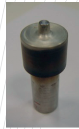
Figure 5 Tool made of steel č.4751
