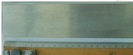
Figure 6 Macrostructure of alloy 6082-T6 (AlMgSi1Mn)
