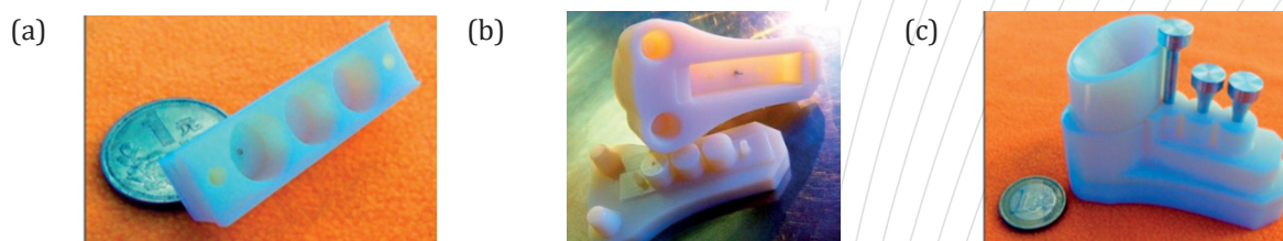
Figure 3 (a) RP master model for sensor cover; (b) & (c) Rapid prototyped mould segments for sensor cover.
