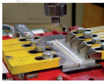
Figure 8 Machine performing FSW
