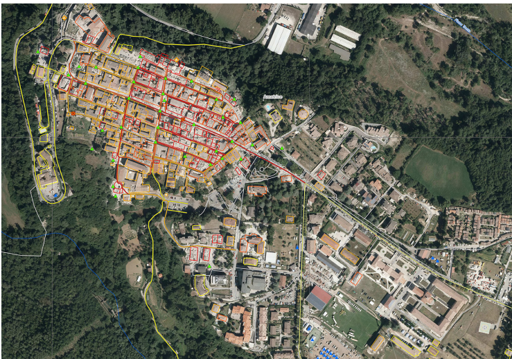
Figure 1. Destroyed (red) and highly damaged (orange) buildings in Amatrice, 25 August 2016.
