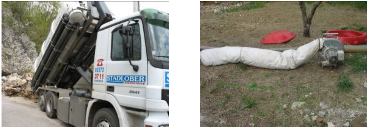
Figure 57: Transporting wood pellets with a cistern (left), ventilator and filter for pneumatic transport (right)
