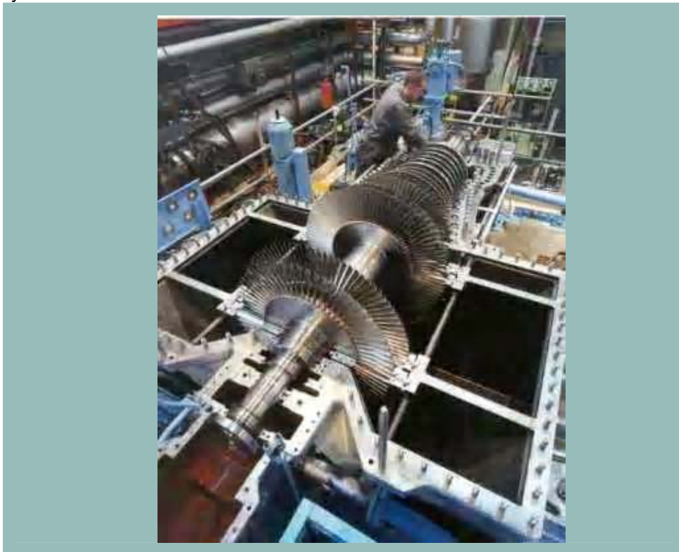
Fig.4.5 - Rotor of a steam turbine with 8 MWeI (Source: Peter Brotherhood Ltd)
