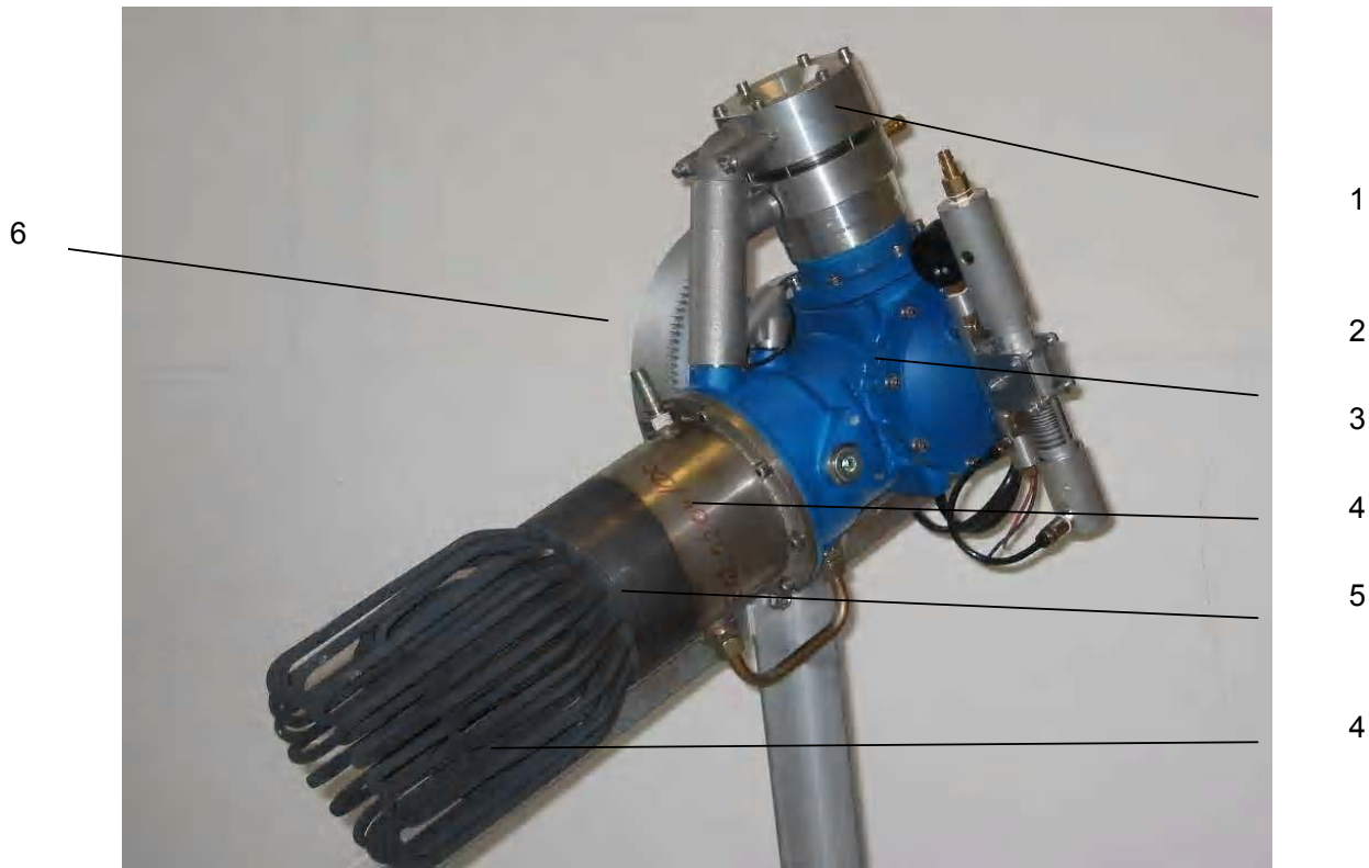
Figure 3.14: 1 kW Biomass gamma type Stirling engine (courtesy of Comp. ENERGIEBIG, Innsbruck, Austria)
