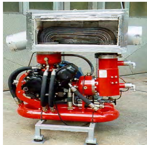
Fig. 1. Biomass Stirling engine at JOANNEUM RESEARCH, Graz, shaft power of 3 kW
