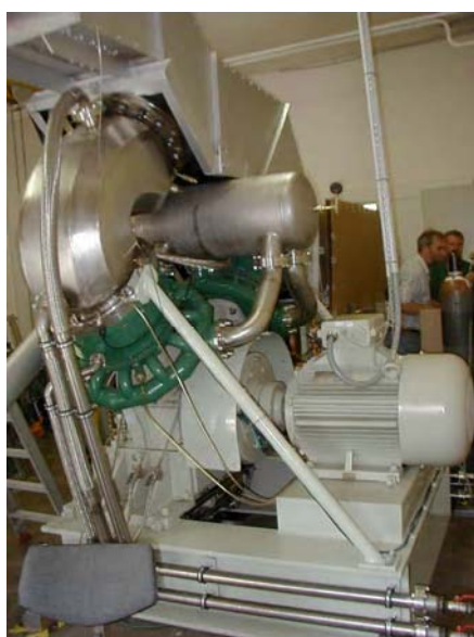
Fig. 6. 30 kW biomass Stirling engine under test at JR.
