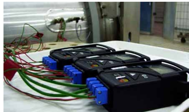
Recording temperature regime of canned meat sterilization
